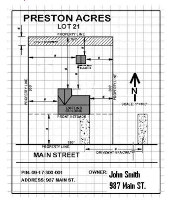
This is an example of the type of information needed on a plot plan.
