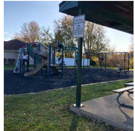
There is not an accessible route or transition to play area
