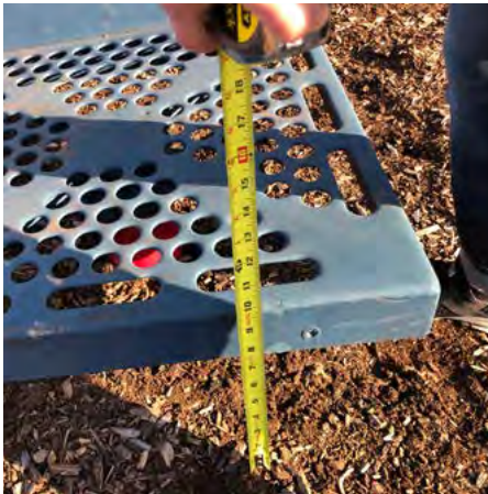
Transfer platform measured approx. 10" above surface
